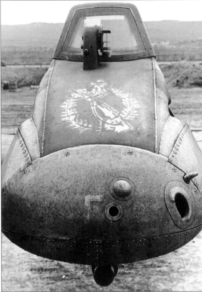
As well as the black triangle on the fuselage, many Hs 129s also displayed the infantry assault badge stencilled on the nose panel ahead of the external Revi C 12/C reflector sight
